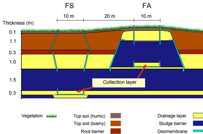
**Figure 1. Layer design of the test fields.**
