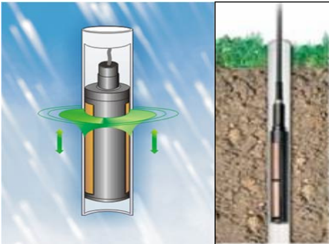
Figure 1. TDR Trime-FM3 probe for borehole moisture measurements. Picture from the site of the IMKO Company.
