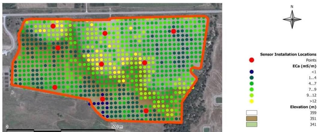
Figure 3. Map showing shallow (0-30 cm) apparent electrical conductivity, field elevations, and a set of targeted soil water monitoring locations.
