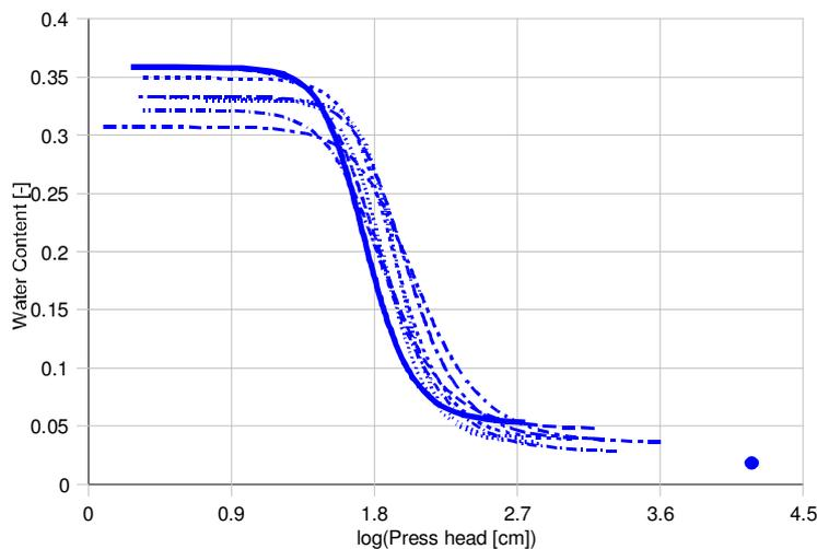
**Figure 2. Best fit van Genuchten function curves for the equilibrium retention points for the 0-10 cm. Sodosol (solid line) and inverse modelling results for the 7 different desorption runs (broken lines). Dot marks the measured 1500 kPa retention point.**
