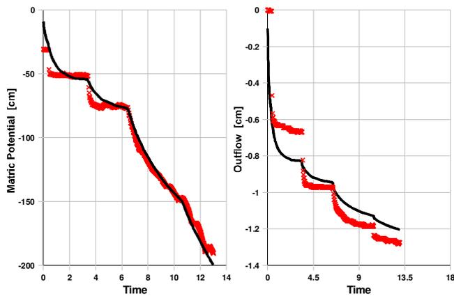
**Figure 1. Measured matric potential and outflow (red markers) and the inverse modelled values (black lines) for the 0-10 cm Red Sodosol.**
