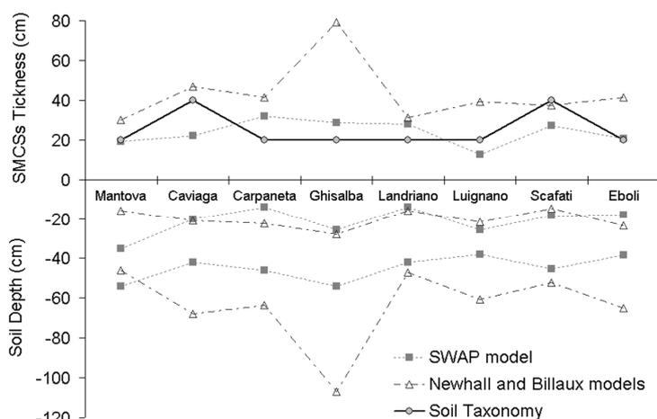
**Figure 2. Upper: SMCS thickness of the eight soil samples according to SWAP (square), Newhall and Billaux (triangle) models, and Soil Taxonomy (circle). Lower: upper and lower boundaries of the SMCS determined using the SWAP model (square) and the Newhall and Billaux models (triangle).**
