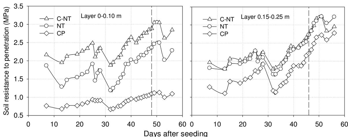
**Figure 2. Variation of the soil resistance to penetration at different compaction levels. The vertical line indicates the time at which the soil moisture (Figure 3) decreased beyond the domain of the soil resistance to penetration estimate functions. CP = chisel plowed; NT = no-till; C-NT = compacted no-till.**
