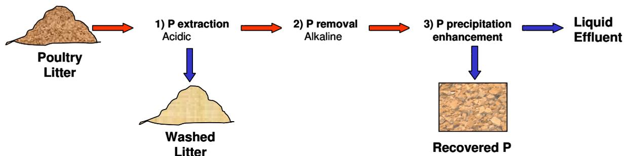
**Figure 1. Quick wash process schematic with steps 1) P extraction, 2) P recovery, and 3) P recovery enhancement.**
