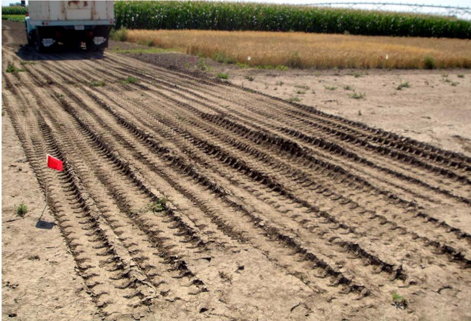
Fig. 2. Wheel tracks from a farm truck during the compaction process in a clay loam soil.
