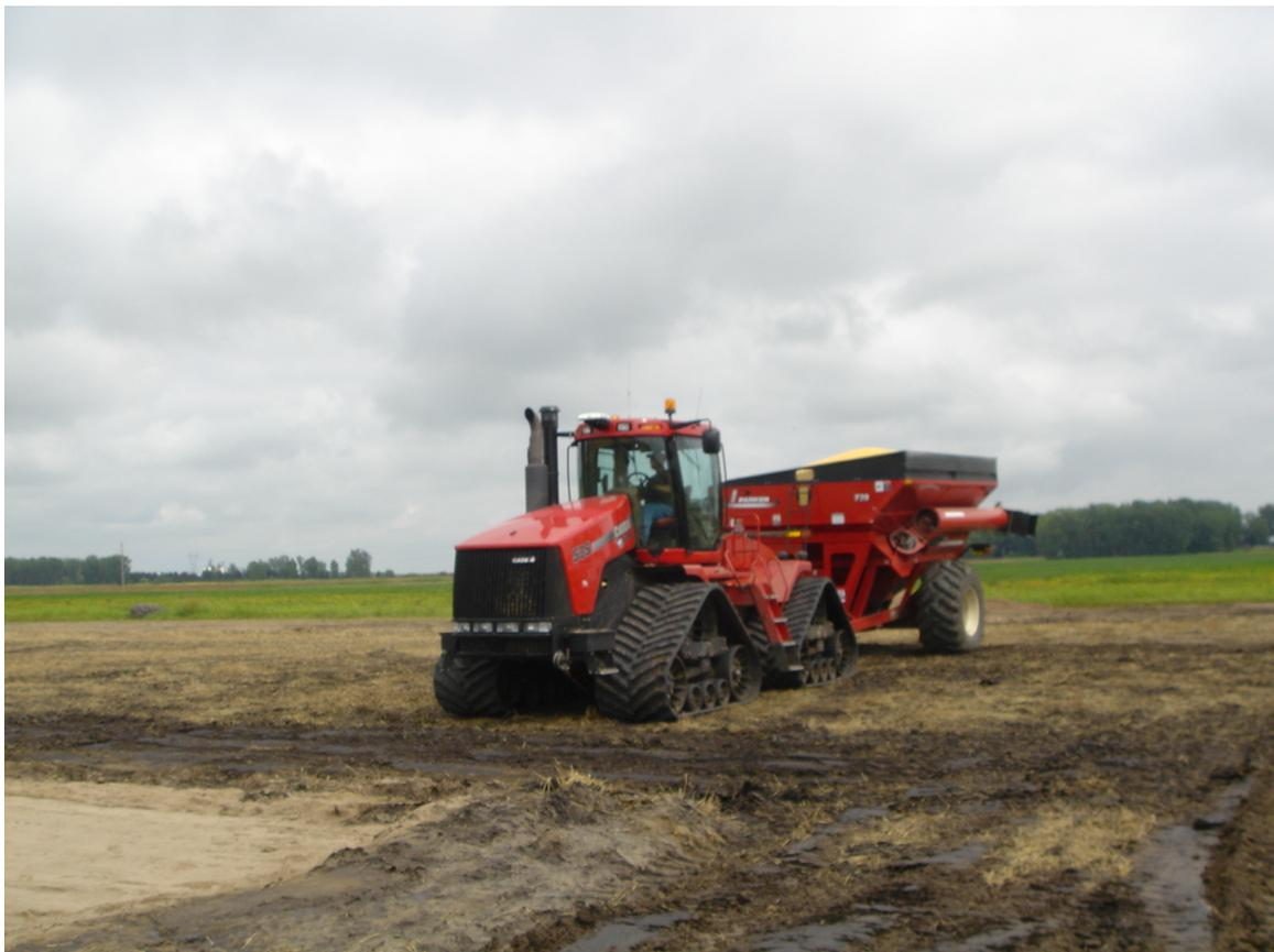
Fig. 1. Soil Compaction caused by heavy machinery under wet field conditions.
