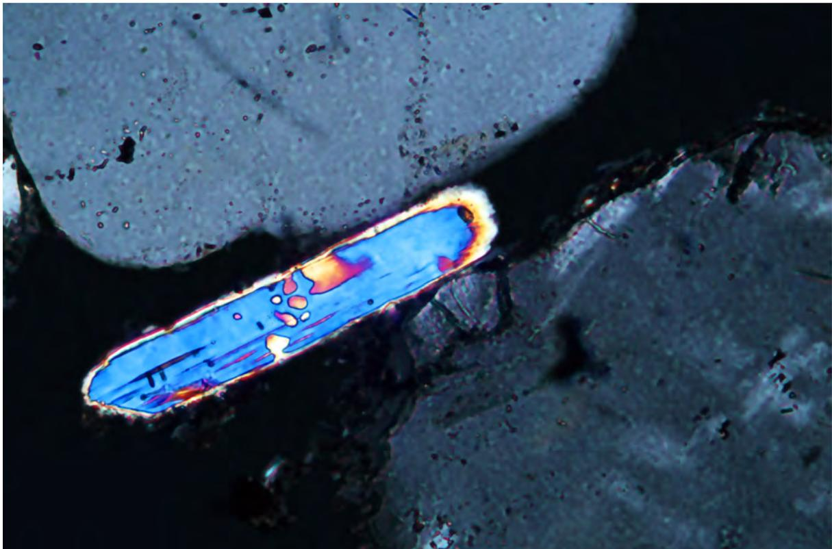
A single mineral of muscovite between two grains of quartz in soil, Field of view: 500  $\mu\text{m}$
