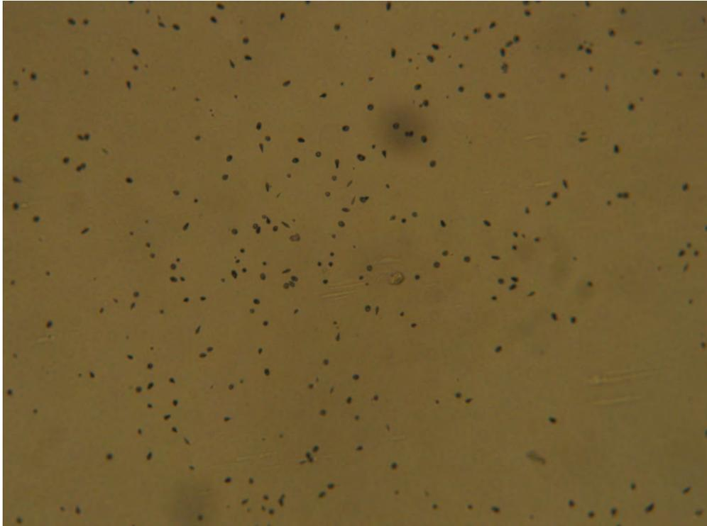
Fig 1 – Alpha track distribution in the clay matrix of a soil with 2-2,5 ppm of Uranium from Campiglia Marittima , Livorno ,Italy
