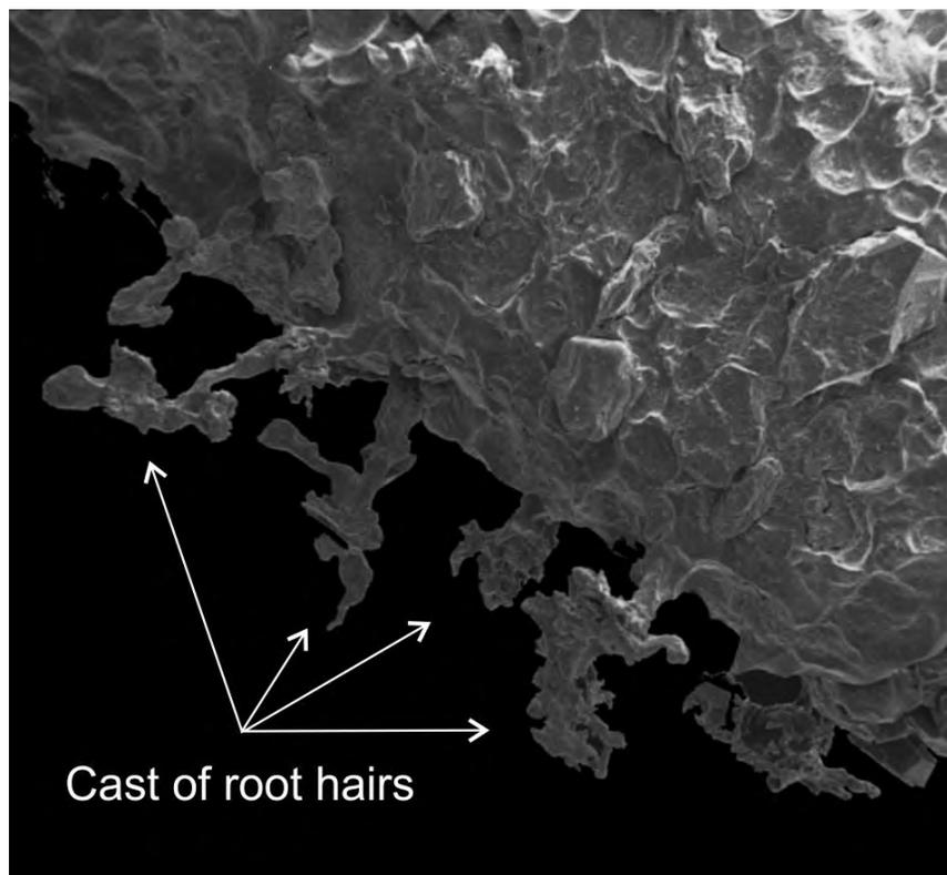
**SEM image of soil pore from 6,000 to 8,000 years old loess by a grass root with casts of root hairs. Field of view 300 microns**
