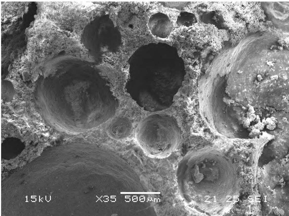
**SEM image of vesicular pores in an Av horizon (i.e. McFadden et al., 1998) beneath a desert pavement in Death Valley, CA, USA (unpublished, Brenda Buck).**
