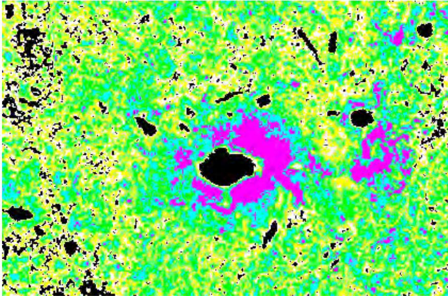
This picture shows the compaction of an undisturbed silty loam in the surrounding of pores caused by grassroots. Pores = Black; Dense areas are represented by darker colours (pink). Field of view: 3.5 mm.
