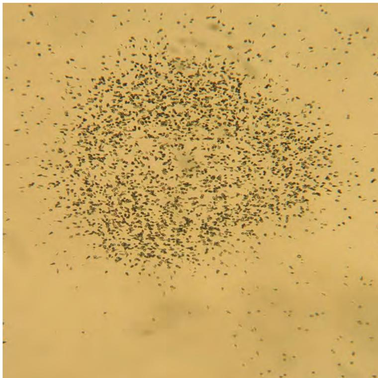
Fig. 2 - Alpha cluster of a soil concretion of the Terra Rossa near Conversano, Murge plateau , Bari, Italy. The approximate Uranium content of the whole concretion is 0,22 Bq /kg
