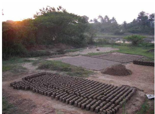
Figure 5 – Sunset on traditional production of bricks from fine alluvial soils
