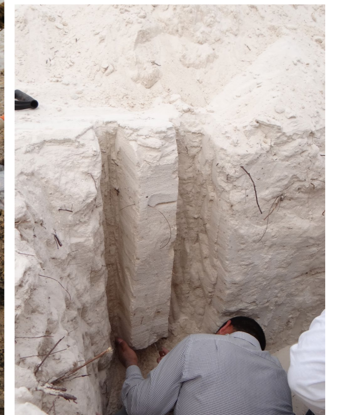
Figure 1 (left): Sampling cores for micromorphology Figure 2 (right): Obtaining the monolith profile in Gypsum Dunes (both: © Marcin Switoniak)
