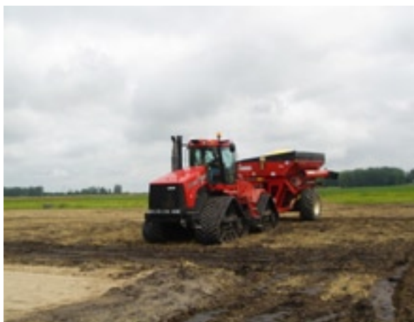
Fig. 1. Soil Compaction caused by heavy machinery under wet field conditions.
