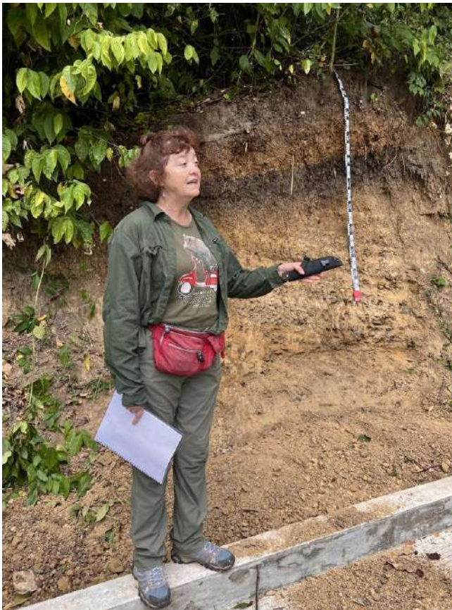
A welded (polygenetic) Greyzemic Phaeozem (Solimovic) over Cambic Phaeozem (Prototechnic, Protovertic) in the vicinity of the archaeological site Palenque explained by Eizabeth Solleiro Rebolledo. Photo courtesy: C. Kabala
